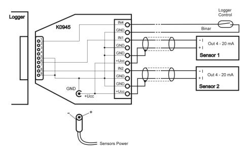
In this case it is possible to power current loop e.g. from ac/dc adapter, connected via coaxial power connector to adapter K0945. Power voltage level depends on applied transducer type.
