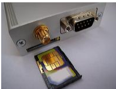
The way to install the SIM card
