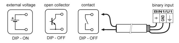
The maximal length of binary inputs and external Pt1000 temperature probe (H4531R only) is 10 m. Connect probe cable shielding to proper terminal and do not connect it to any other circuitry and do not ground it.
