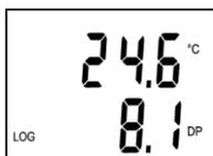
Every 5 s display is automatically switched to displaying of other measured or calculated quantity. Logger now displays ambient temperature and dew point temperature (LCD line marked by symbol DP).
