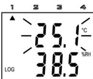
Active alarm is indicated (if display is ON) by blinking of the value of proper quantity on the display and arrow symbol appears at the LCD upper side at the same time. Arrow 1 indicates active alarm for ambient temperature, arrow 2 relative humidity and arrow 4 dew point temperature.
