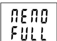
If measured value is out of the measurable or displayable range numeric reading is replaced by hyphens. If memory is totally full filled in non-cyclic logging mode, logger is switched OFF and message MEMO FULL appears on the LCD. It appears also if logger is operated with switched OFF display.
