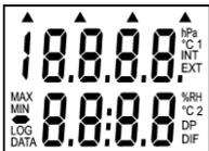
After switching ON the instrument all symbols on the LCD are displayed for about 2 seconds.
