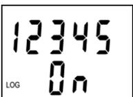
**If LCD is switched ON**, actual readings are displayed then – counter value on the upper line (with respecting of optional user recalculation to real input quantity). Lower line displays binary input actual state. Symbol On indicates closed contact (respectively low voltage level), symbol OFF indicates opened or not connected contact (respectively high voltage level). Symbol LOG indicates logging in progress – if it blinks, data memory is filled for more than 90%.
